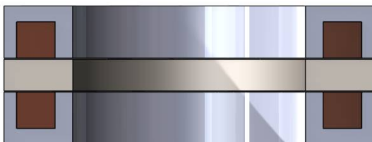
Fig. 3: Thrust bearing configuration with a single coil and two poles on each side of the thrust disk.
